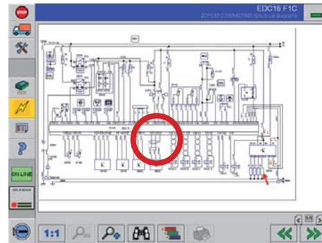
The position of the selected component is indicated on the connection diagram by a **red arrow**
