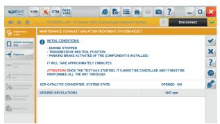
ARD Exhaust gas aftertreatment system, system reset.
