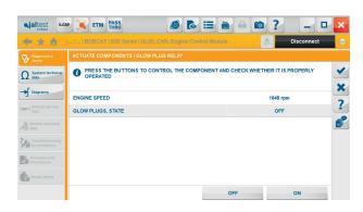
• New DL03 system in Doosan engines that includes functions such as heaters activation or fuel metering valve test.
