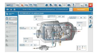
System Display of Eberspächer auxiliary heater system.
