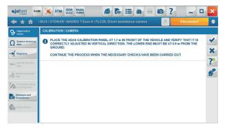
• New ADAS systems, FLR21 radar and FLC20 camera. Both systems, which are installed in numerous vehicles such as OTOKAR buses, FORD Cargo trucks, etc., include system calibrations.
