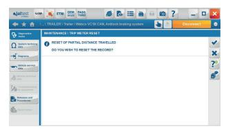
ABSVCSII braking system, partial distance travelled reset.
