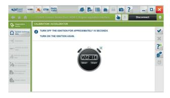
During the execution of some functionalities, it is necessary to wait a certain period of time until performing any operation. From this version, in this type of steps, Jaltest offers a countdown timer with the set time.
